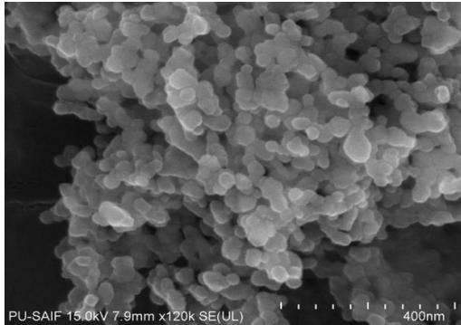
**Figure 2.** FESEM image of Ag-ZnO nanoparticles
